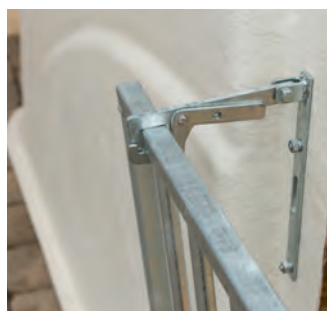
Side guards stop calves from slipping through and lend stability
