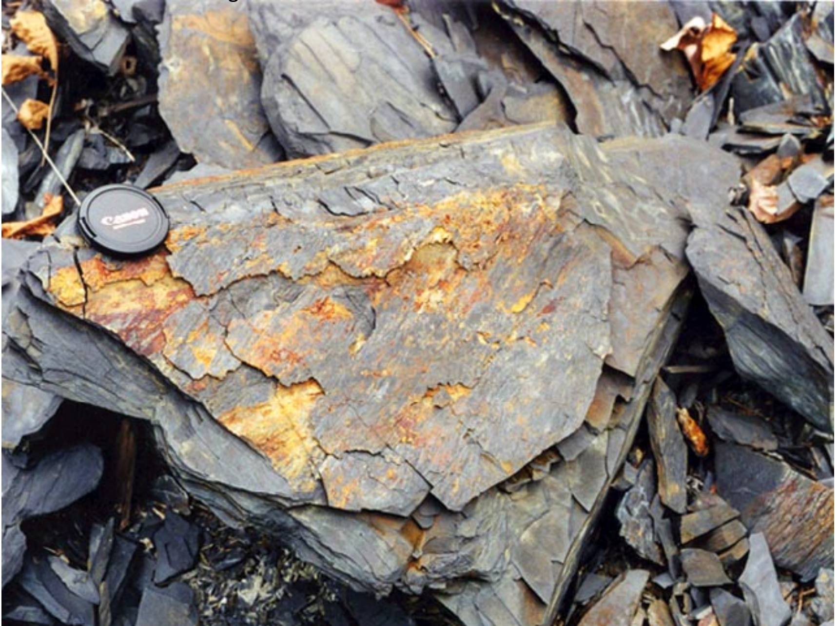
Oxidation of Fe-bearing minerals in shale
