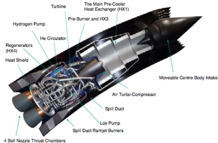
Figure 6. SABRE cutaway<sup>11</sup>
