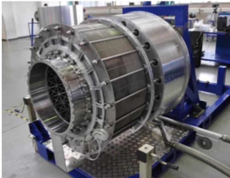
Figure 14. Full sized pre-cooler on the test stand.<sup>9</sup>
