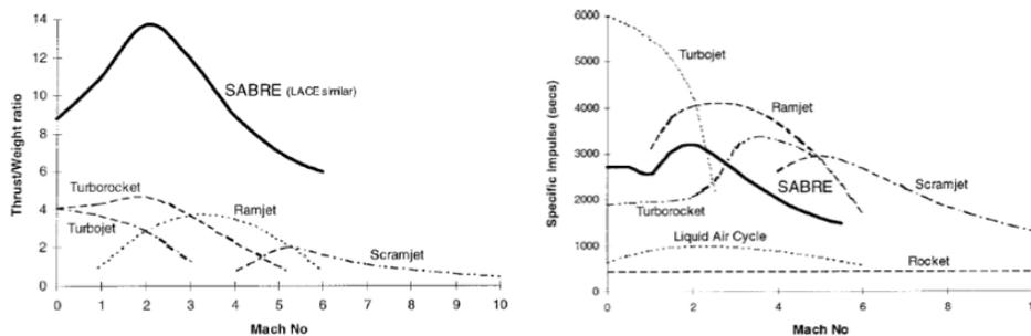
Figure 13. SABRE comparisons to other classes of engines.<sup>11</sup>
