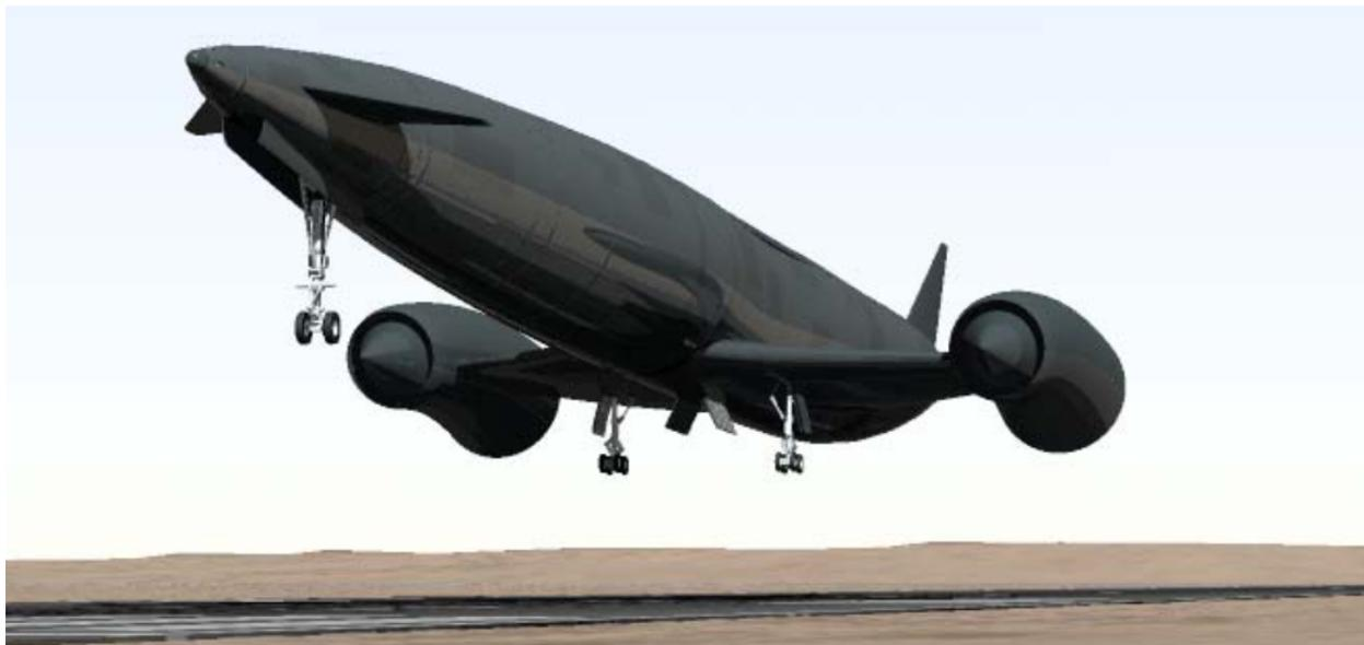
Figure 5. Visualization of SKYLON undercarriage deployed for landing.<sup>1</sup>
