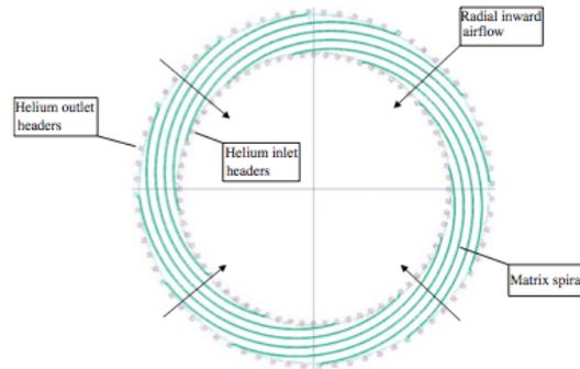
Figure 9. Pre-cooler flow diagram.<sup>16</sup>
