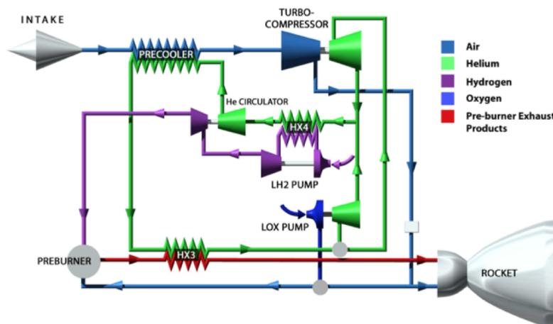
Figure 7. SABRE system schematic<sup>11</sup>
