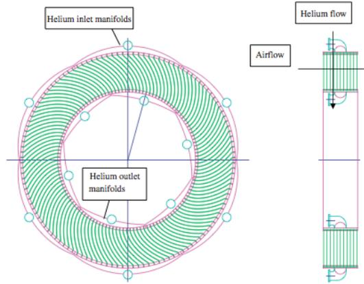
Figure 11. Helium flow in pre-cooler.<sup>16</sup>
