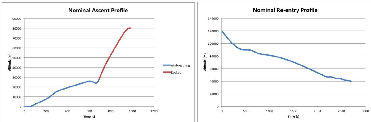
Figure 2. Ascent and Re-entry profile for equatorial launch.<sup>3</sup>
