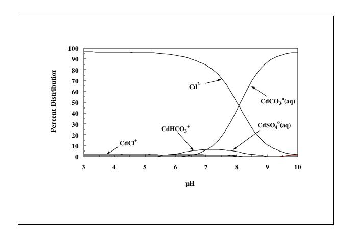
**Figure 5.1**. Calculated distribution of cadmium aqueous species as a function of pH for the water composition in Table 5.1. [The species distribution is based on a concentration of 1 micro g/l total dissolved cadmium and thermodynamic data supplied with the MINTEQA2 geochemical code.]
