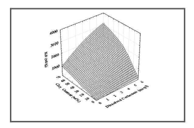
**Figure G.2**. Variation of  $K_d$  for plutonium as a function of clay content and dissolved carbonate concentrations.
