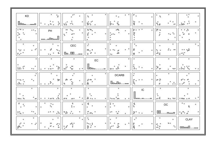
**Figure G.1**. Scatter plot matrix of soil properties and the distribution coefficient (K<sub>d</sub>) of plutonium.
