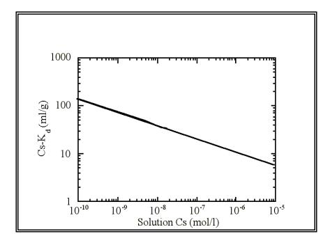
**Figure D.5**. Cesium K<sub>d</sub> values calculated from generalized Freundlich equation (Equations D.3 and D.4) derived from the literature.
