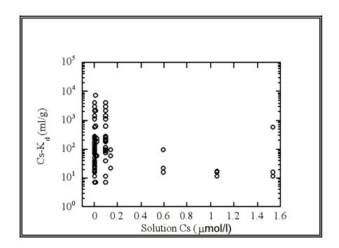
**Figure D.3**. K<sub>d</sub> values calculated from an overall literature Freundlich equation for cesium (Equation D.2).
