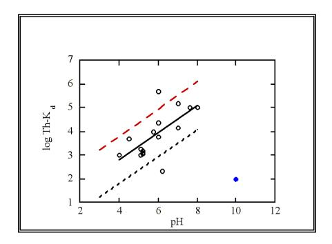
Figure I.2. Linear regression between thorium  $K_d$  values and pH for the pH Range 4 to 8. [Values  $\pm 1$  logarithmic unit from the regression line are also identified. The single  $K_d$  value at pH 10 is identified by the filled circle)].
