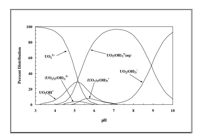
Figure 5.6b. Calculated distribution of U(VI) hydrolytic species as a function of pH at  $1,000~\mu g/l$  total dissolved U(VI). [The species distribution is based on U(VI) dissolved in pure water and thermodynamic data from Wanner and Forest (1992).]
