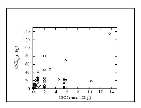
$\label{eq:figure H.2.} Figure \ H.2. \quad \text{Relation between strontium $K_d$ values for soils with CEC values less than $15$ meq/100 g.}$
