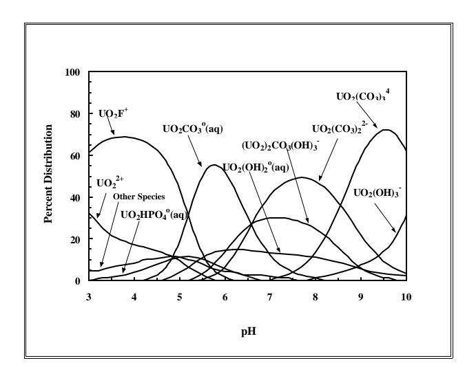
Figure 5.7. Calculated distribution of U(VI) aqueous species as a function of pH for the water composition in Table 5.1. [The species distribution is based on a concentration of 1,000 μg/l total dissolved U(VI) and thermodynamic data from Wanner and Forest (1992).]
