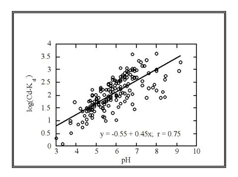
Figure C.1. Relation between cadmium K<sub>d</sub> values and pH in soils.
