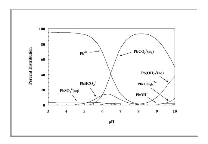
**Figure 5.2.** Calculated distribution of lead aqueous species as a function of pH for the water composition in Table 5.1. [The species distribution is based on a concentration of 1 micro g/l total dissolved lead.]
