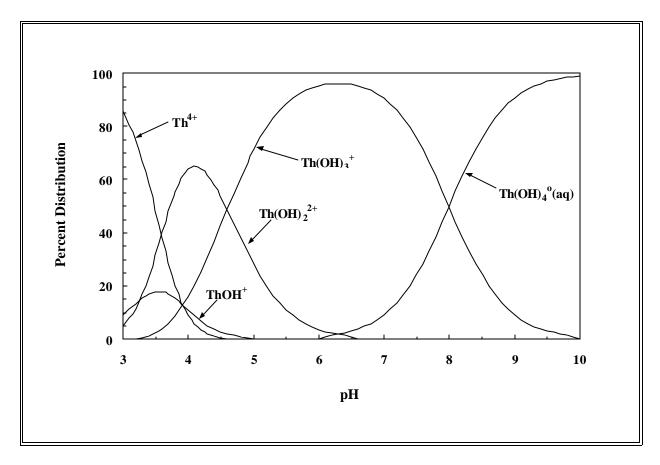
**Figure 5.4.** Calculated distribution of thorium hydrolytic species as a function of pH. [The species distribution is based on a concentration of 1 micro g/l total dissolved thorium in pure water (*i.e.*, absence of complexing ligands other than OH) and thermodynamic data from Langmuir and Herman (1980).]
