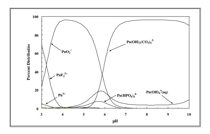
**Figure 5.3.** Calculated distribution of plutonium aqueous species as a function of pH for the water composition in Table 5.1. [The species distribution is based on a concentration of 3.2 x 10<sup>-10</sup> mg/l (1.36 x 10<sup>-15</sup> M) total dissolved plutonium.]
