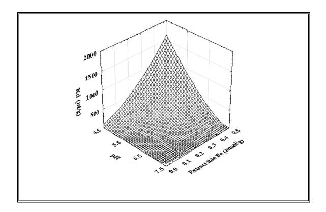
**Figure E.1**. Variation of  $K_d$  for Cr(VI) as a function of pH and DCB extractable iron content without the presence of competing anions.
