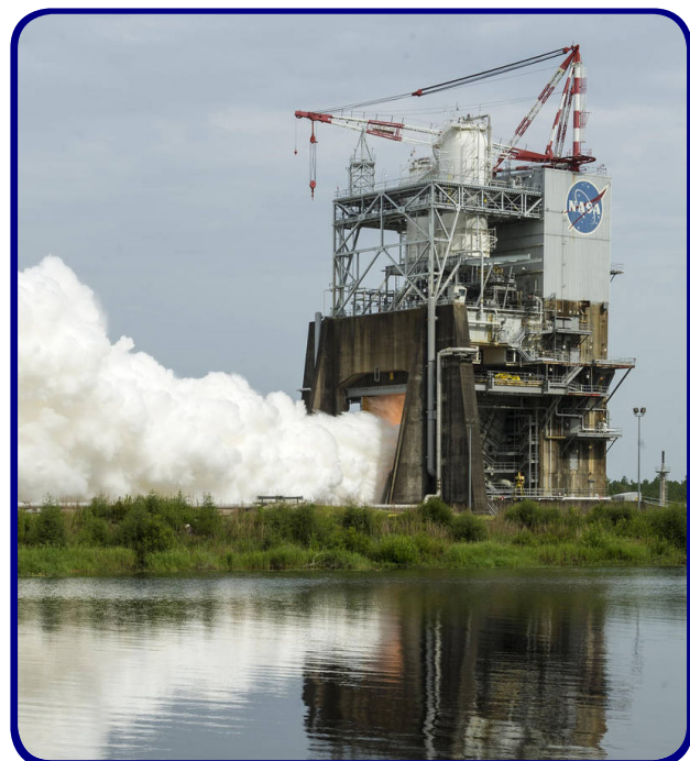
Image Caption: Engineers conducted an SLS RS-25 rocket engine test fire at NASA's Stennis Space Center, Mississippi, in June 2015. (Credit: NASA)
