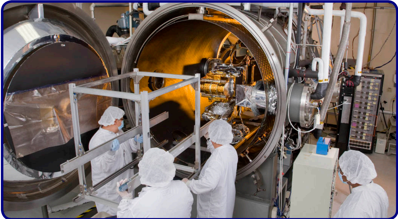
Image Caption: Engineers prepare to remove the CERES instrument from the Radiometric Calibration Chamber following the completion of thermal vacuum testing at Northrop Grumman's manufacturing facility in Redondo Beach, Calif. This sensor will be integrated onto NOAA's JPSS (Joint Polar Satellite System) spacecraft, scheduled for launch in 2017. (Credit: Northrop Grumman Corporation)
