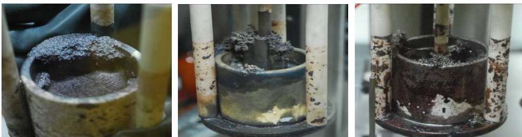
Figure 8: The shapes of the uranium dendrites formed on the cathode crucibles after electrodeposition tests were conducted at 200 mA/cm 2
