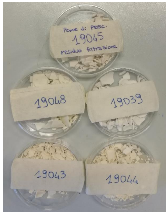
Fig. 31 Recovered material after precipitation and drying (number 19045 refers to sample "SGO (2)", 19048 to sample "Zurich", 19039 to sample "SGO (1)", 19043 to sample "Karlsruhe" and 19044 to sample "S. Rocco I").
