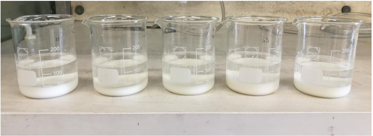
Fig. 30 Suspension obtained after adding lime milk.
