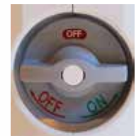
SHUT OFF VALVE
